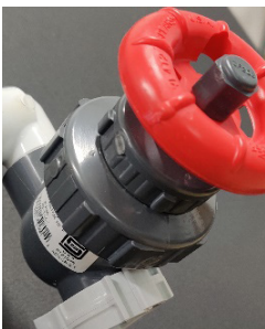
Picture 8 Flow control valve
